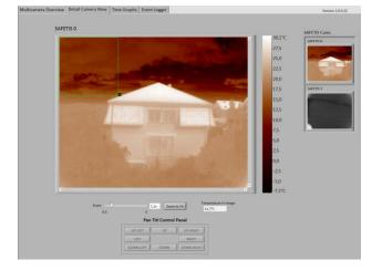
SCU with SDK can disaply all SAFETIS cameras as live thermal streams in real time in tile view. In case of need any SCU could be viewed in detailed window for particular monitoring including visualization of all ROI. With using SAFETIS SDK can be programmed **live graphs** of maximal temperatures in time of all SCU. Application events log is also available where all the alarms, connections, disconnections or logins are listed with exact date and time.
